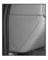
The fuse block access door is on the driver's side edge of the instrument panel. Pull off the cover to access the fuse block.
